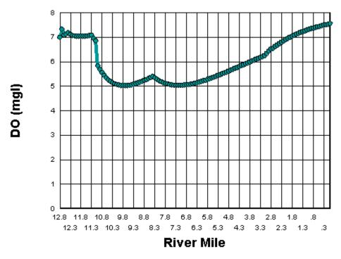
Figure 15. Model Output for DO in Snake Creek, Maximum Load Scenario
