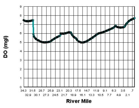
Figure 14. Model Output for DO in Bakers Creek, Maximum Load Scenario
