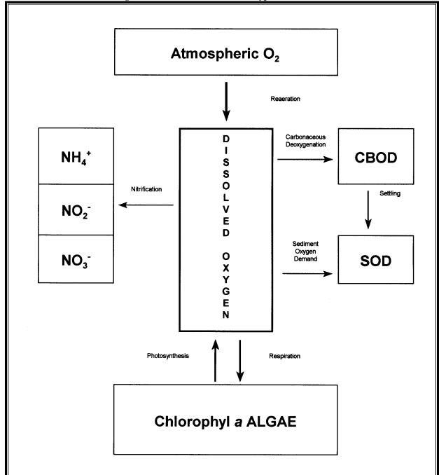
Figure 6. Instream Processes in a Typical DO Model
